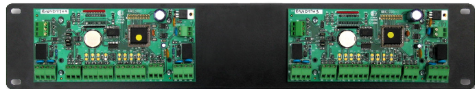
NURC-2005 includes two URC-2003-B controllers installed on a R2U 19" rack mount plate as shown above.
