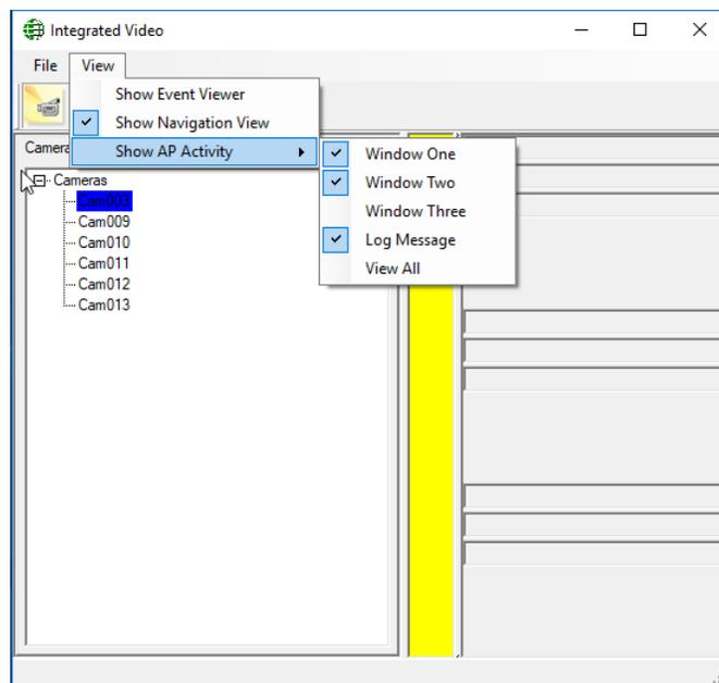
Access Point Activity section displays data pertaining to a specified access point. Three different windows can display data for three different access points. A fourth window (Log Message) will display data from a selected message in the Event Viewer. *Click* to show or hide the applicable window (one, two, or three), or the Log Message window. *View All* will restore the section to show all four windows, or if all four are already showing it will hide the whole section.
