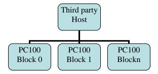
Each PC100 can be assigned a block of 256 inputs according to the following table:
