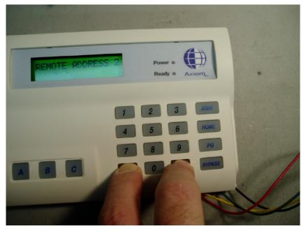
To change the address, hold the \* and # buttons down for about 3 seconds.
