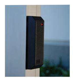
Installation The MM-6800 reader is designed to fit perfectly on the 1-3/4 inch standard metal door frame or window mullion. The metal-compensation that is built into every MM-6800 reader assures minimal loss of read range when the reader is mounted on a metal surface. The MM-6800 reader also can be fastened by 2 screws on any wall or other surface. Installation may be indoors or outdoors, exposed to weather.
