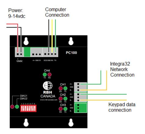
The PC-100 connects to the IRC-2000 through the RS-485.
