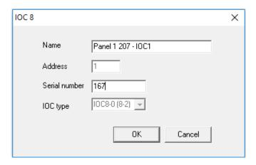
Enter each device's individual serial number, as labelled on the board. There are two types of IOC8's available; eight inputs, two outputs (8-2); and four inputs, four outputs (4-4).
