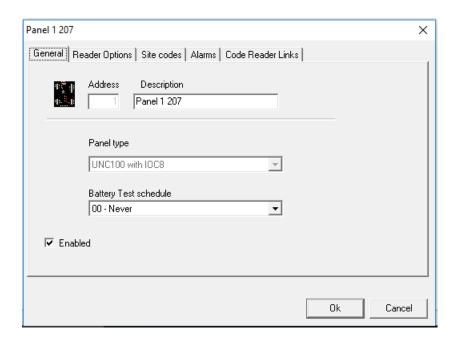
The option to add IOC8 is available only when the panel is configured as UNC100 with IOC8 in software.
