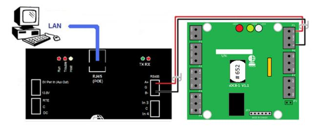
The IOC8 is wired into the UNC100's RS485 port with a two conductor shielded cable.
