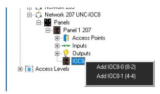
Only 1 panel per network can be added when using UNC100 with IOC8.
