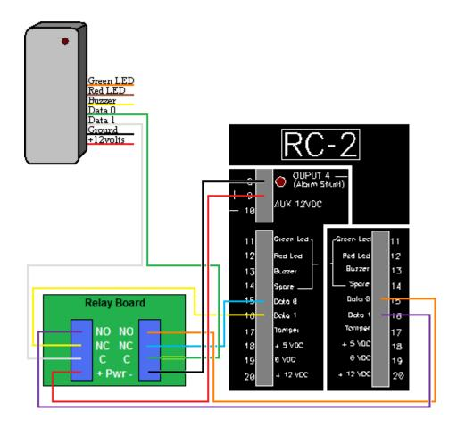
• Relay board connection helps to switch the second cardholder swipe on the reader connected to side A to show as a swipe on side B, so that the pictures of both the cardholders can be seen on the video screen at the same time. This is achived with global command explained later.
