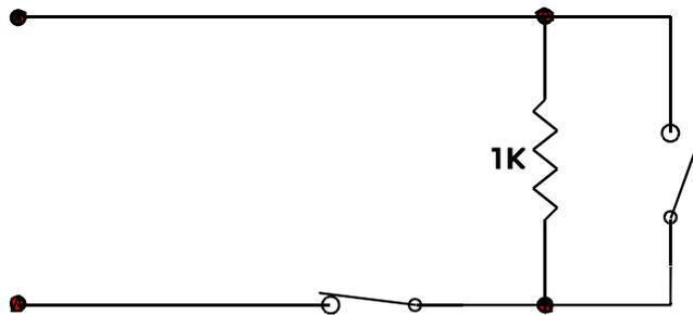
This circuit type is used where normally open and normally closed contacts are used in the same loop.
