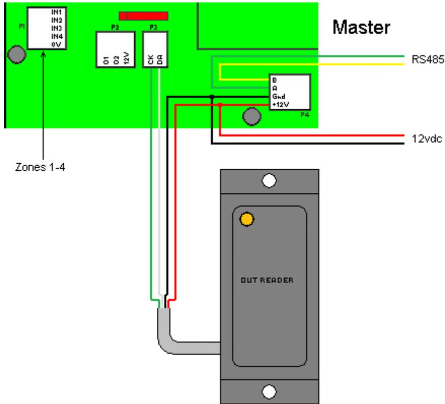
Only four wires from the reader are connected; Data0, Data1, and two for power. On the RBH-AXS-LCD-4z panels connect Data0 and Data1 to terminal CK and DA.
