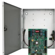
NIRC-2000-B Controller is designed for mounting in the standard ENCL-1-PS enclosure. LEDs and DIP switch bank are mounted on the front of the controller board.
