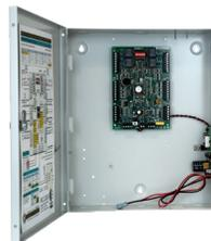
NIRC-2000 includes one NIRC-2000-B controller installed in an ENCL-1-PS enclosure
