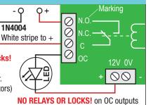
\* Functionality of relay polls will be reversed vs. printed marking
