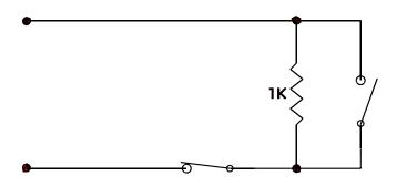
This circuit type is used where normally open and normally closed contacts are used in the same loop.
