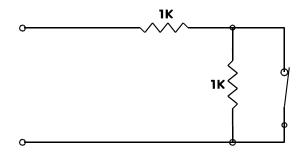
This circuit provides a high degree of supervision and detects both short and open circuit fault conditions. Use this circuit in high security applications.
