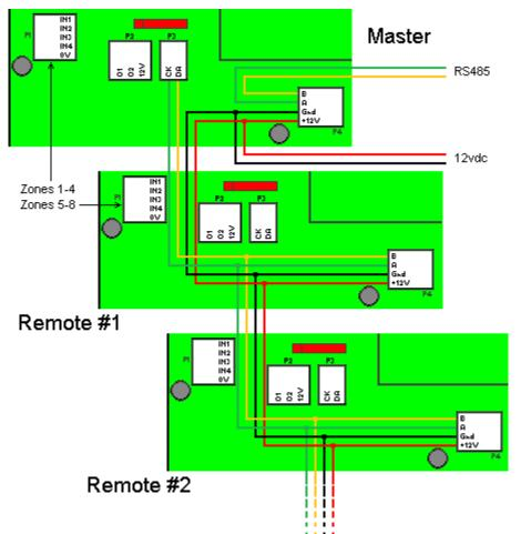
Connect terminal CK on the master keypad to A of all remotes. Then connect terminal DA on the master keypad to B of all remotes.
